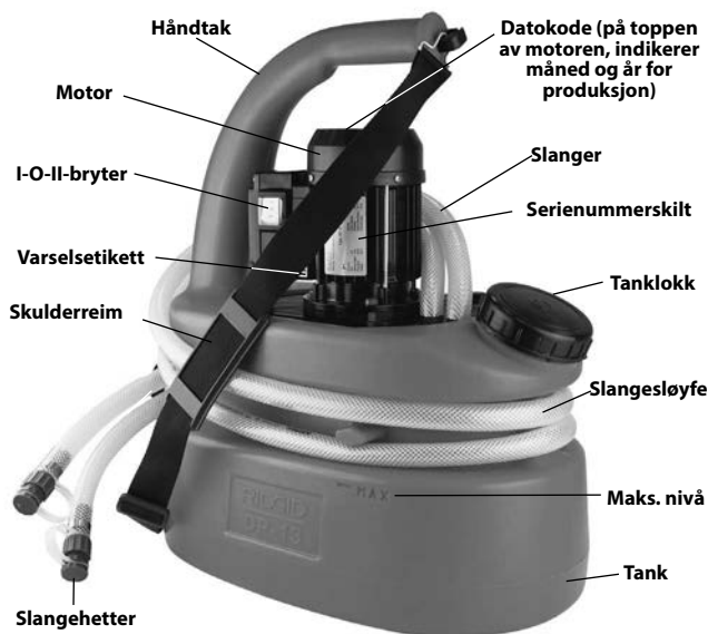
Figur 1 – RIDGID DP-13 Avkalkingspumpe
