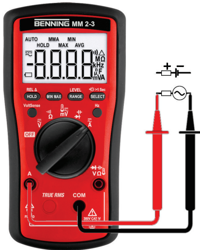
Figure 10: Current or frequency measurement
