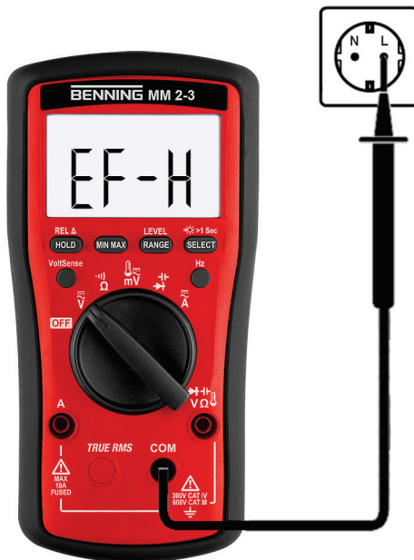
Figure 15: External conductor or phase testing
