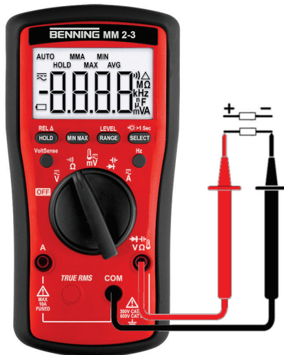
Figure 11: Resistance measurement or continuity test
