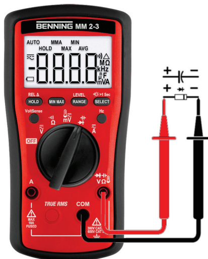
Figure 12: Capacitance measurement or diode testing
