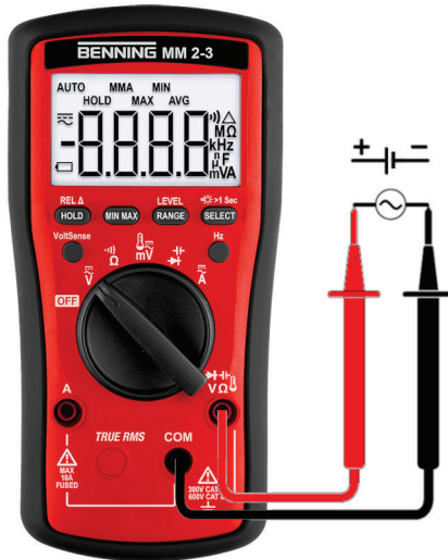
Figure 9: Voltage or frequency measurement
