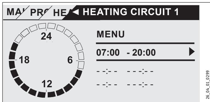
You can set three switching time pairs per day or block of days. The switching time pairs are shown on the display, to the right of the clock. Each switching time pair consists of a start time and an end time.
