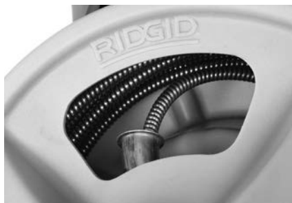
Figure 18 – Coil Cable Into Drum As Shown
