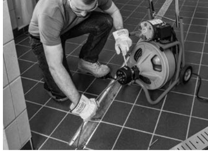
Figure 15 – Operating K-400 with AUTOFEED
