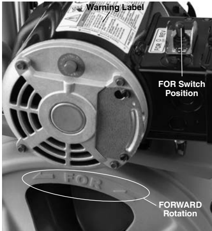
Figure 8 – Proper Drum Rotation (FOR Switch Position)
