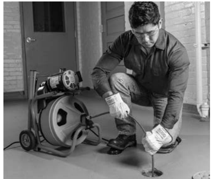
Figure 13 – In Operating Position, Manually Feeding Cable
