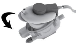
**EN** The sump/detection unit must be cleaned and serviced at regular intervals in accordance with the degree of pollution existing within the pump operating environment.
