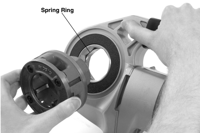
Figure 9 – Installing Die Heads into 600-I Power Drive
