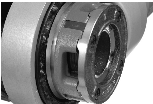
Figure 15 – Pipe Even with Edge of Dies
