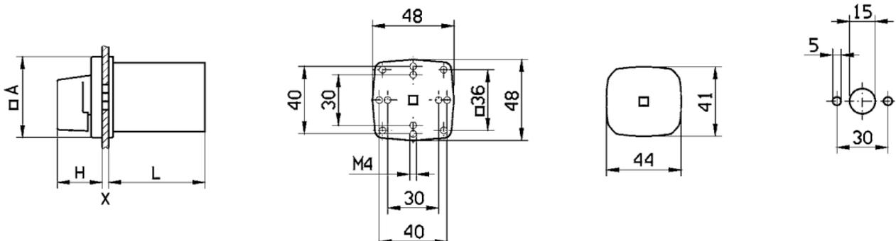
A=48mm, H=27mm, Xmax=4mm, L=33mm
