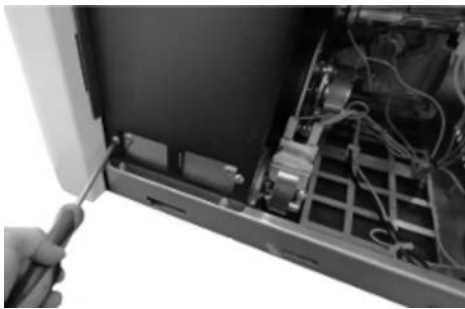
Fig. 78 - Reinigung Raumventilator (Atena 3 Plus 12/14 - Duke 12/14 At - Saba 12/14)
