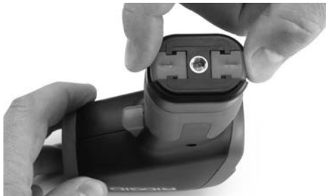
Figure 4 – Removing Battery Compartment
