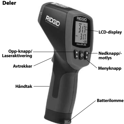
Figur 2 – mikro IR-200, deler
